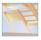
It is particularly important to ensure that the vapour barrier is fastened to the beams and adjoining gable walls so that it is air-tight.
