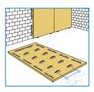
Daubs should be approx. 100 mm in size and the gaps in between approx. 300 to 400 mm on Rigidur boards being used as a substrate for ceramic coverings e.g. tiles.
